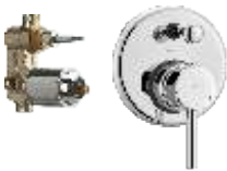
High flow single lever concealed diverter system consisting of Exposed part (lever, tip ton knob, flange) and Concealed part (45 mm cartridge with button assembly, cartridge sleeve) Exposed part F2004721 ₹ 1825 Concealed part F4030101 ₹ 3880 Set ₹ 5705
