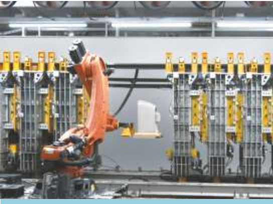
Sanitaryware Robotic Pressure Casting Machine - For producing clone type product every time
