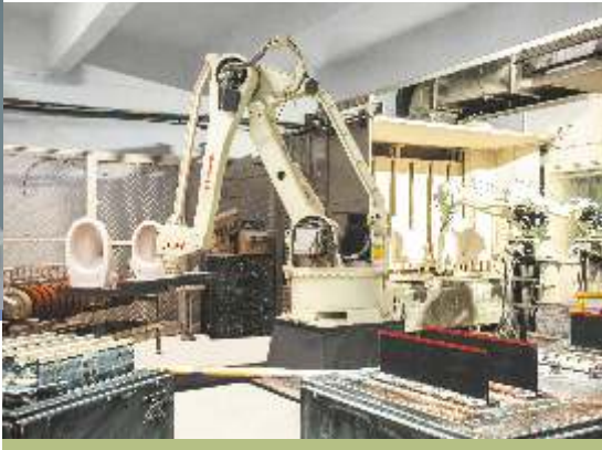
Sanitaryware Robotic Glazing - For uniform glazing ensuring smooth surface
