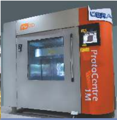
Sanitaryware 3D Printer - For making quicker prototypes of new designs
