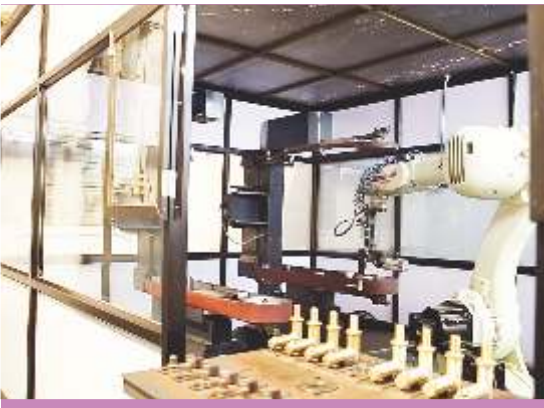
Faucet Robotic Surface Grinding - Helps in uniform coat of chromium plating that will lead to surface endurance
