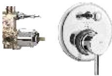
5-way (3 inlets + 2 outlets) single lever concealed diverter system consisting of Exposed part (lever, tip ton knob, flange) and Concealed part (cartridge with button assembly, cartridge sleeve) Exposed part F2004711 ₹ 1630 Concealed part F4020101 ₹ 3755 Set ₹ 5385
